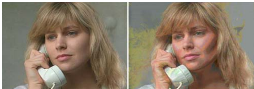
Avivo 12-bit Analog-to-Digital conversion (left) vs. low quality 9 or 10 bit ADC
