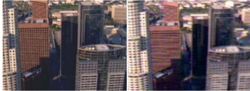
Avivo 3D Comb filtering (left) vs. typical 2D comb filtering (right – note color bleeding on brown buildings)
